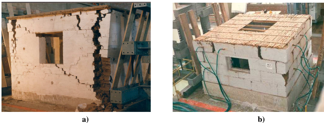
Figure 1 – Experimental tests of unreinforced earthen models: a) adobe house, b) rammed earth house (credits: [Zegarra, L. et al.; 1997])
