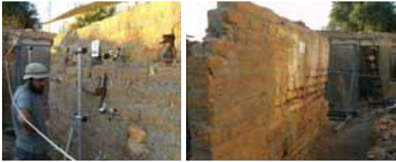
Figure 6. In situ out-of-plane cyclic testing layout: wall; horizontal displacement transducers; and horizontal loading system.
