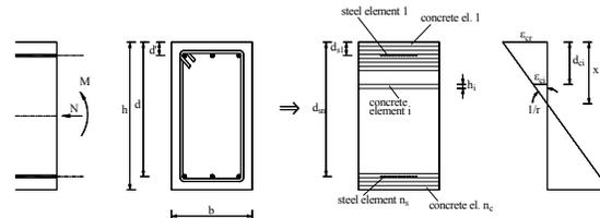
Fig. 3. General fibre model for RC elements
