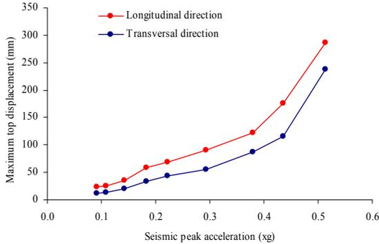
Fig. 16. Top displacement vs. seismic peak acceleration
