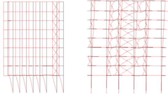
Fig. 10. Natural vibration modes ( $f_{1,X} = 1.08\text{Hz}$  and  $f_{1,Y} = 1.75\text{Hz}$ )
