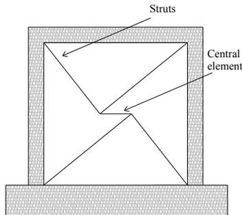
Fig. 5. Infill masonry panel macro-model
