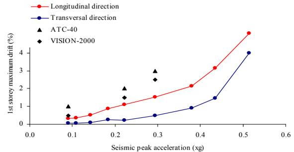
Fig. 17. 1<sup>st</sup> storey drift vs. peak earthquake acceleration and safety limits
