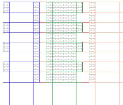
Fig. 8. Equivalent structural system for transversal direction (Y)
