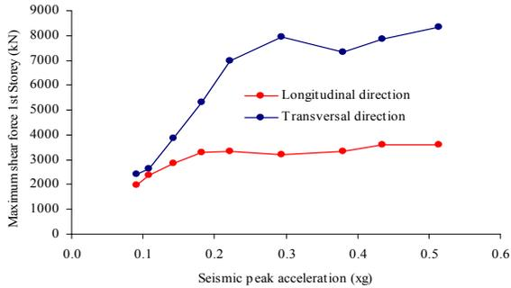
Fig. 15. 1<sup>st</sup> storey shear vs. seismic peak acceleration
