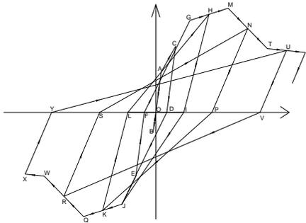
Fig. 6. Hysteretic model for infill masonry panels [Rodrigues et al., 2005]
