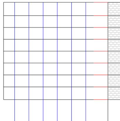
Fig. 9. Equivalent structural system for longitudinal direction (X)
