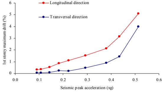
Fig. 14. 1<sup>st</sup> storey drift vs. peak earthquake acceleration
