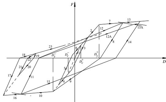
Fig. 4. Hysteretic model for RC elements [Varum, 1996]
