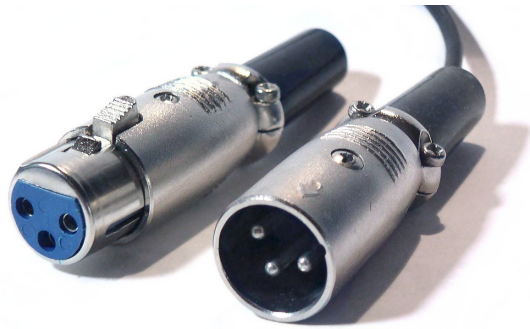
Figure 2.4: Female (left) and male (right) 3-pin XLR connectors.
