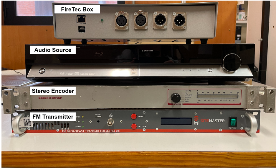
Figure 4.11: Devices used to assemble a setup to emulate an FM radio station.
