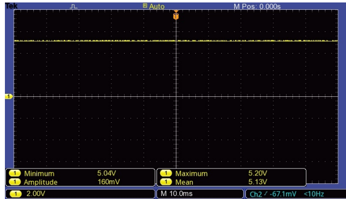
Figure 4.4: Oscilloscope screenshot showing the output of the L7805CV regulator.
