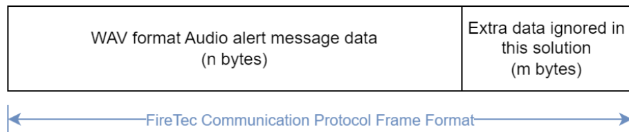
Figure 3.19: Structure of the FCP data frame.
