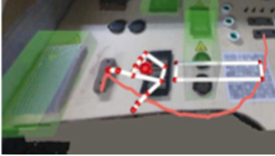
(a) Remote user's view in VR, showing the local user's environment as a colored point-cloud. A representation of the remote user's tracked hand can be seen, which is using a pointing gesture to sketch 3D lines for an arrow. The transparent green areas are dangerous areas already highlighted by the remote user.
