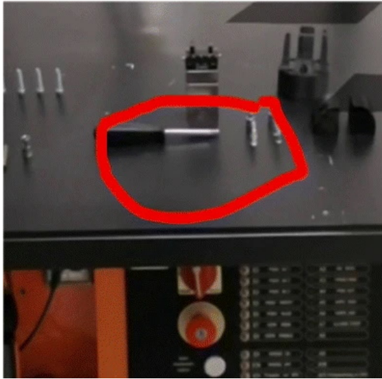
(a) Hand drawing, simply a 2D sketch drawn by the remote user on the screen and temporarily overlaid over it.
