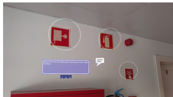
(b) AR side. Note the 3 additional buttons below the comment box, to mark the task as OK/NOK or NA.
