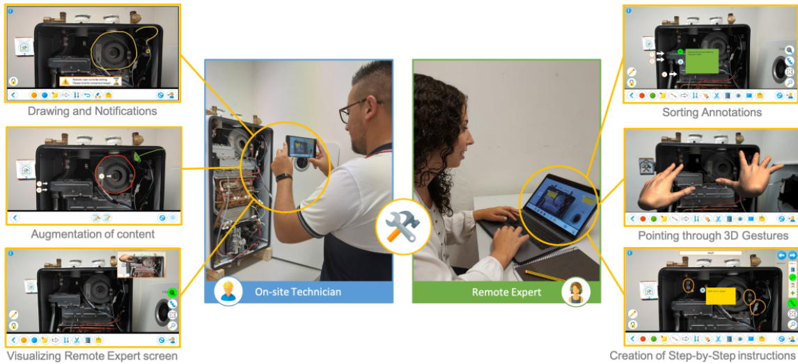
Figure 2.7: Representation of Marques, Silva, Teixeira, et al. 's system [26]. The local user is shown on the left, using a hand-held device to see a AR view of his workspace, while the remote user is shown on the right, creating the AR content in the desktop application. Images and video can be shared between the users, which can then be annotated with 2D objects, which are shared and positioned in 3D in the AR view. 2D sketches, text boxes, arrows, and numbering (sorting) annotations are available, along with other features, such as notifying the local user when the expert is creating new content, gesturing by using hand-recognition, or organizing annotations into step-by-step instructions.
