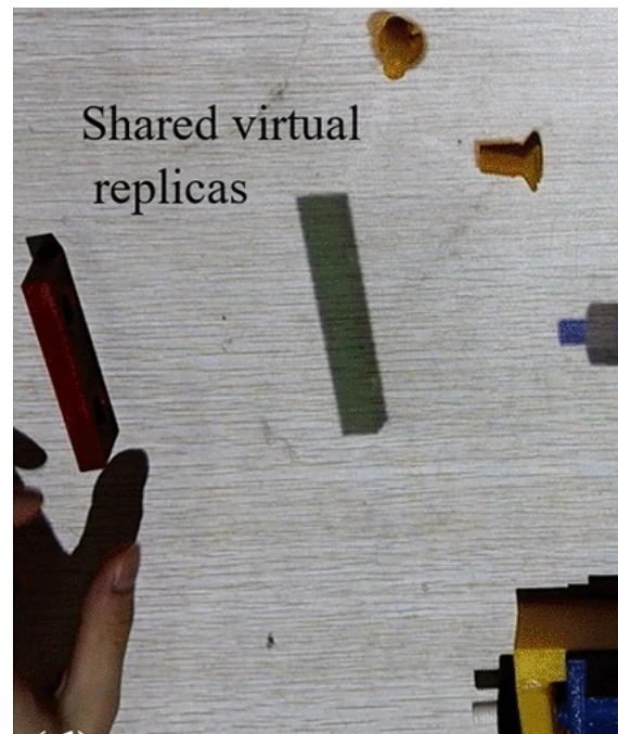
(b) Local user view, with the SAR elements projected on the same table the user is working on the assembly task. Projected virtual replicas can be seen in the center and center-right, and their physical counter-parts on the center-left and top-center, respectively.
