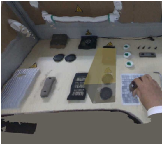
(a) Remote user's view, showing the local user working on the assembly task and an area that was highlighted by the remote user as dangerous (center). This area is initially green and transparent but has already shifted in color and transparency as the local user's hand (to its right) approached it.
