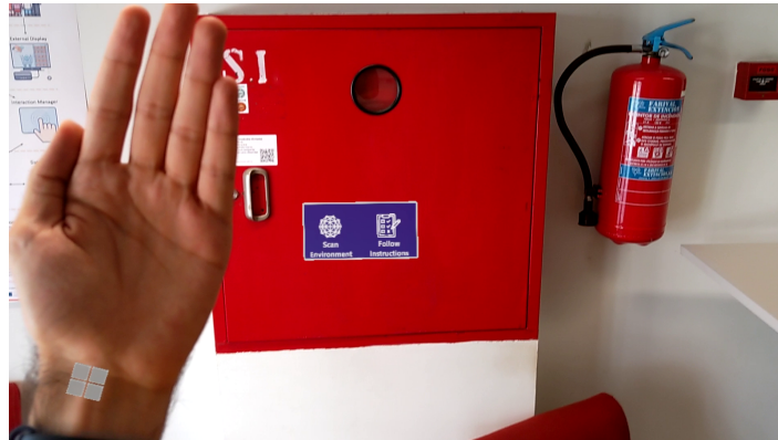
Figure 3.8: Palm gesture being used to open a hand menu, showing the main menu of the application, from which submenus for the environment scan and instruction execution are accessed.
