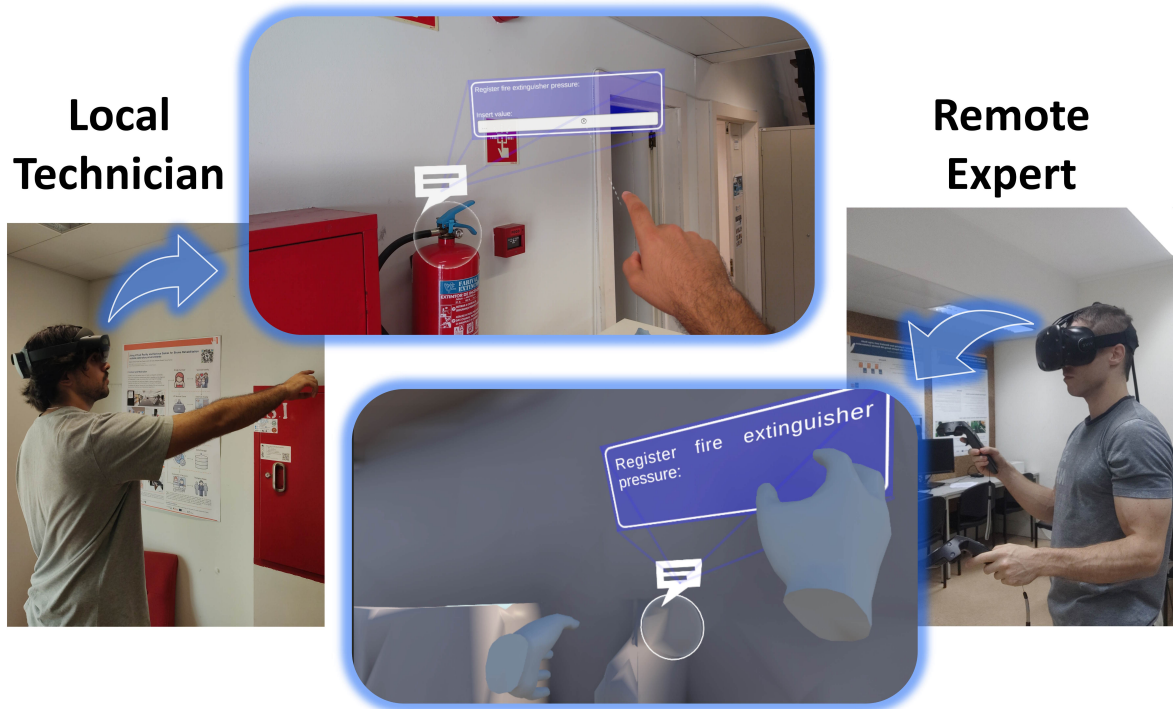
Figure 3.1: The AR (left) and VR (right) applications that comprise the system, used by the local technician on a Microsoft HoloLens 2 and the remote expert on a HTC Vive, respectively.
