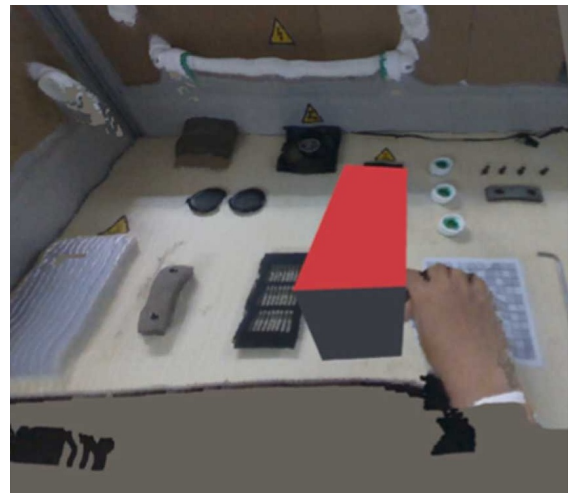
(b) Remote user's view, showing the same highlighted area from (a) after the local user's hand has entered it. The area becomes completely solid and red to notify both users of the danger.
