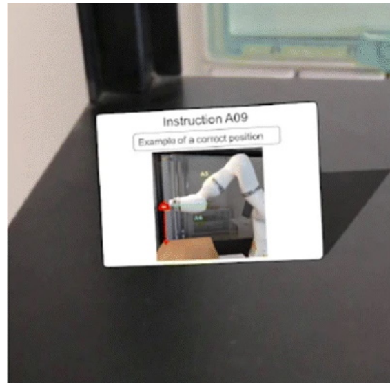
(d) Instruction card containing a GIF, a 2D object positioned by the remote user with 6DOF tracking in the local user's environment.
