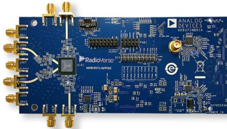
Figure 4.9: ADRV9371-WPCBZ radio card [51].
