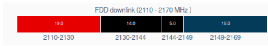
Figure 4.2: 2100 MHz 4G LTE n1 FDD downlink band allocation in Portugal - retrieved from [4].
