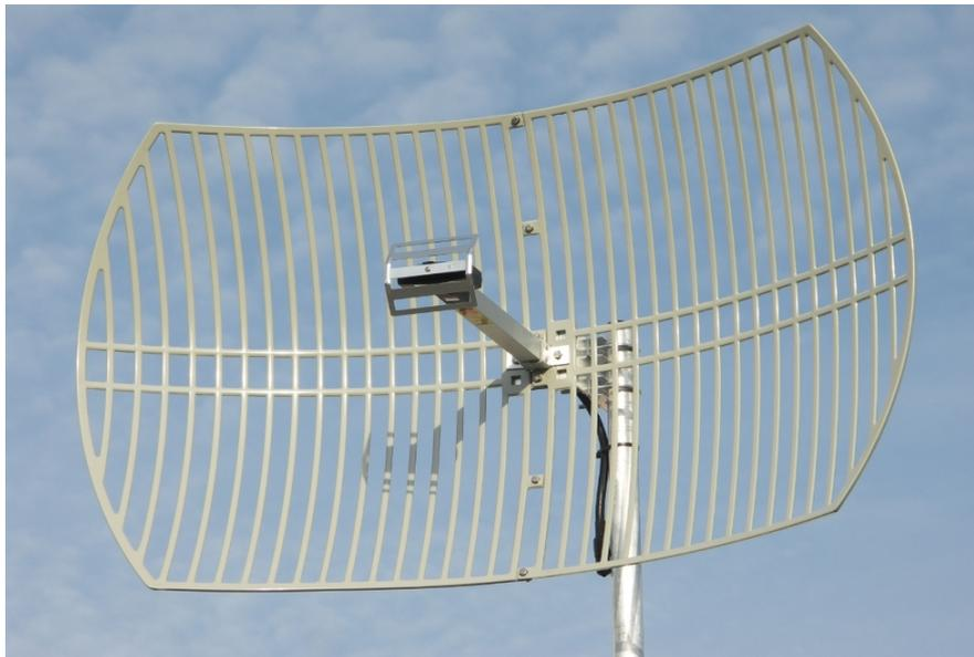
Figura 4.22: Antena *ground segment* 2.4GHz.
