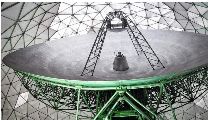
Figura 2.14: TIRA, Space Observation radar, Fraunhofer FHR.
