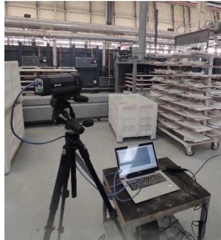
Figure 9. Thermographic camera fixed FLIR A320 Tempstream.
