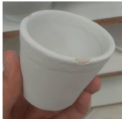
Figure 2. Example of defect in small absences in glazed or glazed chipped.
