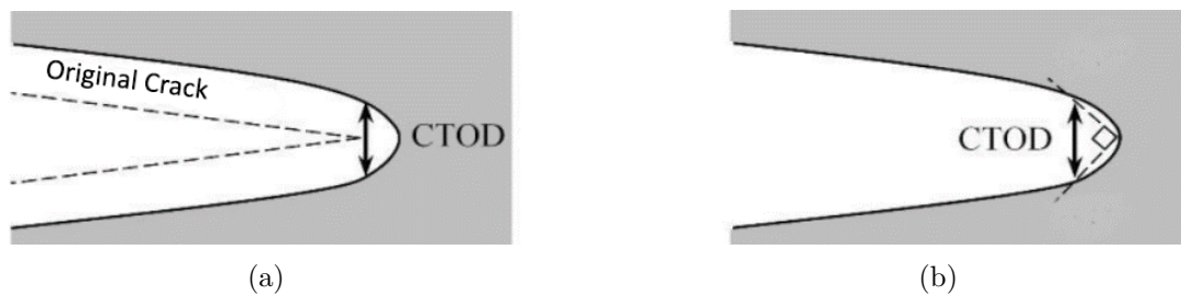
Figure 2.6: Definitions of CTOD: (a) CTOD equal to the displacement normal to the plane of the crack relative to the position of the tip; (b) CTOD equal to the displacement at the intersection of a 90^\circ vertex with the faces of the crack (from [14])
