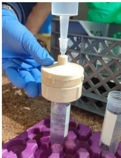
Figure 26: Portable filter unit used during in-situ filtration of CdV water samples.
