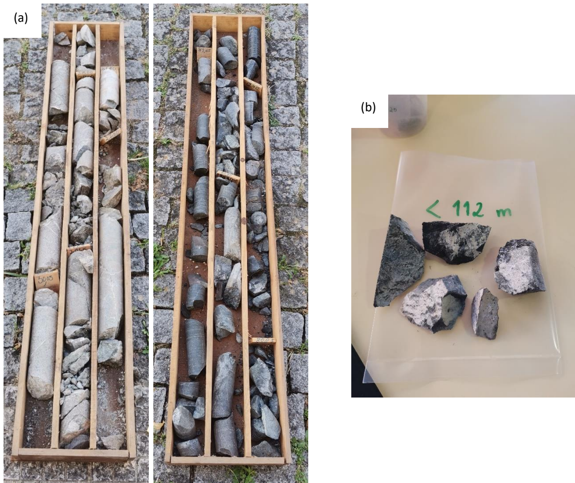
Figure 18: (a) Rock samples used in their core drawers; (b) sample after being broken shows a white layer that represents a fracture vein, that when scratched, turns into a fine dust.
