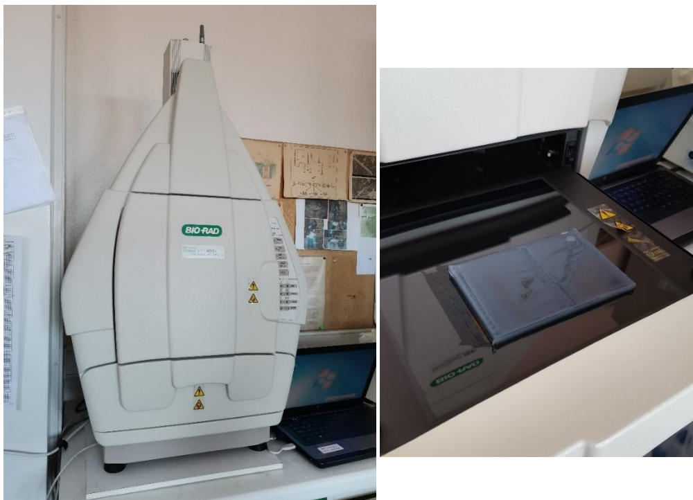
Figure 48: Molecular Imager (left) and final Agarose Gel loaded into the imager (right).
