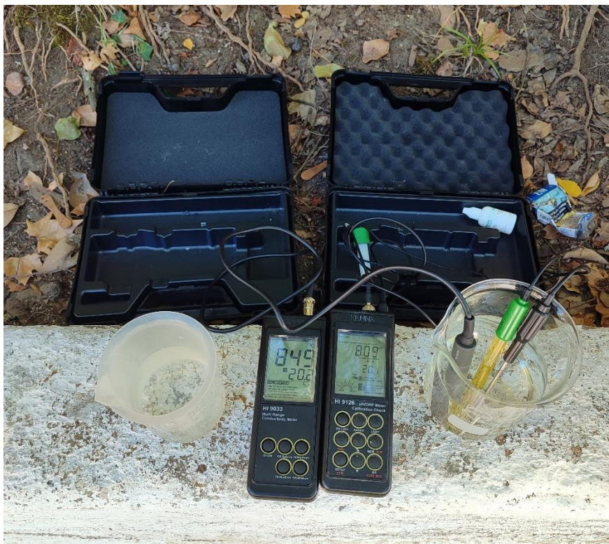
Figure 27: Multi parameters used to measure pH, conductivity, temperature and ORP in-situ.
