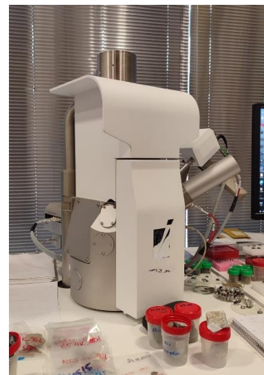
Figure 36: Schematic of a Scanning Electron Microscope (Adapted from http://www.ammrp.orf.au/ ) (left), and TESCAN VEGA SEM used to analyze CdV samples (right).
