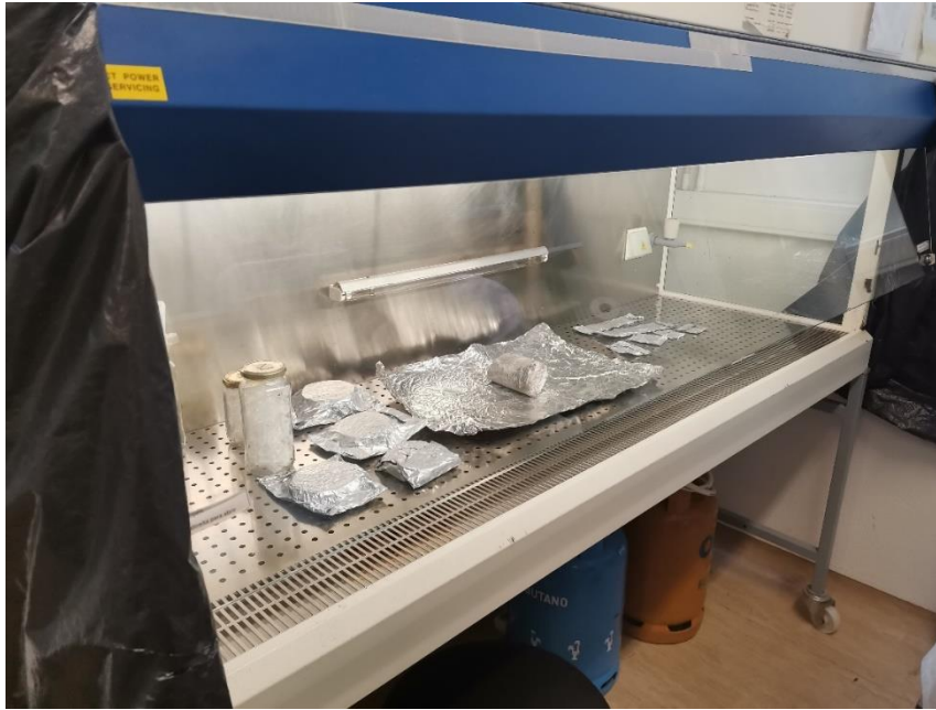
Figure 39: Sample core inside flow chamber ready to be sterilized with UV light and whole equipment used.
