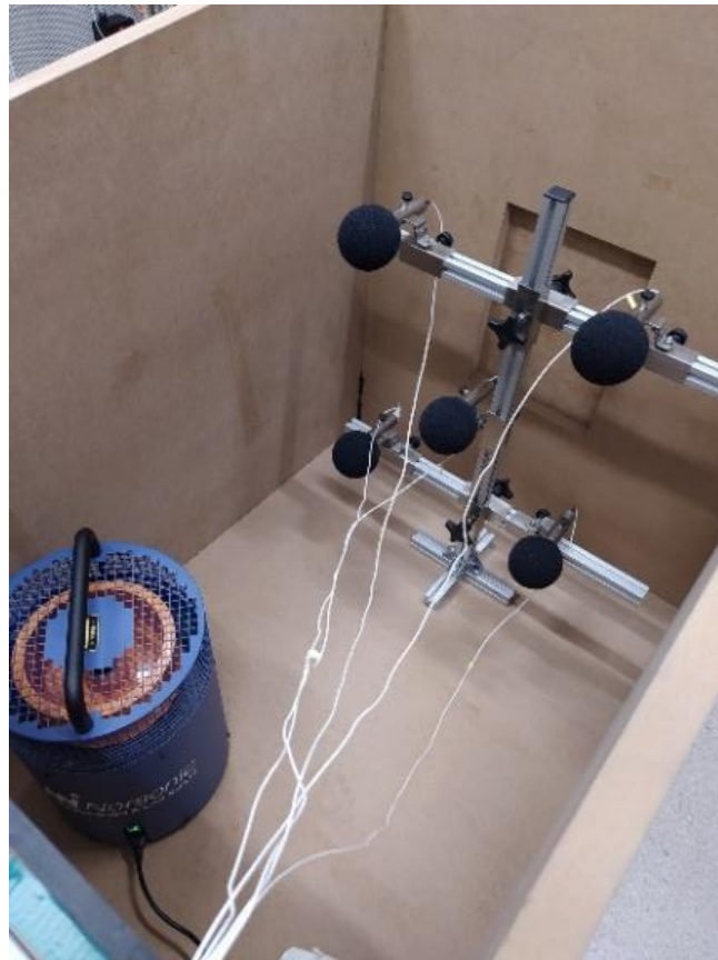
Figure 19 - Validation test setup, mic stand positioned 25 cm away from front wall
