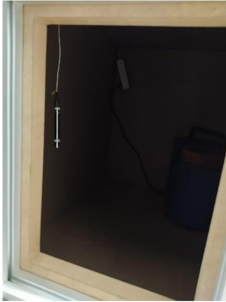
Figure 21 - Single hanging microphone test
