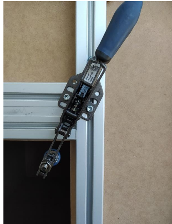
Figure 6 - Toggle clamps used to hold the material sample.
