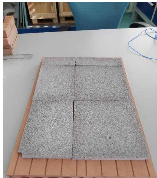
Figure 30 - WPC board fitted with 8 mm geopolymer
