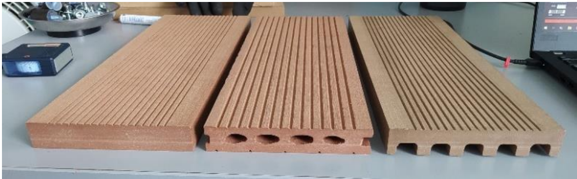
Figure 24 - 3 WPC board types tested
