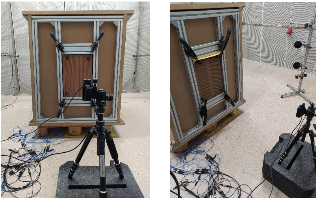
Figure 23 - STL test setup with WPC sample
