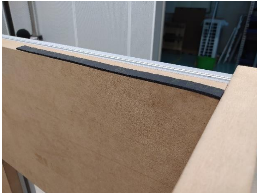
Figure 8 – Foam used to cover air gap.
