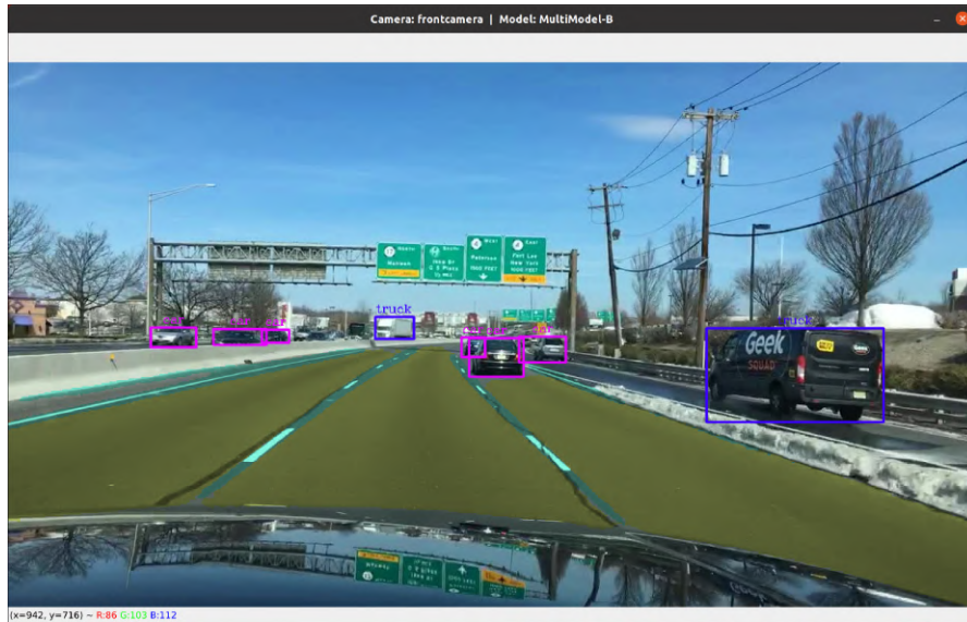
Figure 5.8: Inference output of multiple single-task neural networks: one for object detection, a second one for drivable area segmentation, and a third one for lane marking
