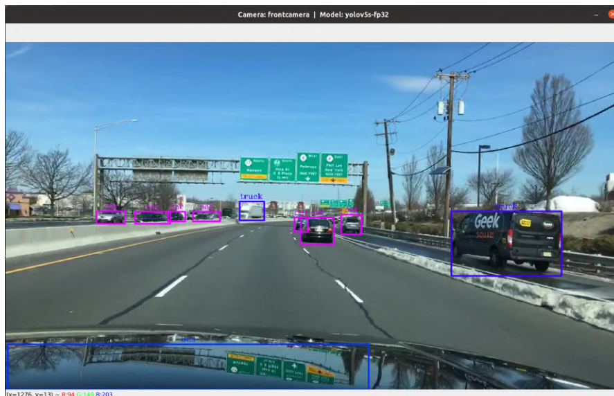
Figure 5.2: Inference output of a single-tasked neural network for object detection. Bounding boxes identify objects
