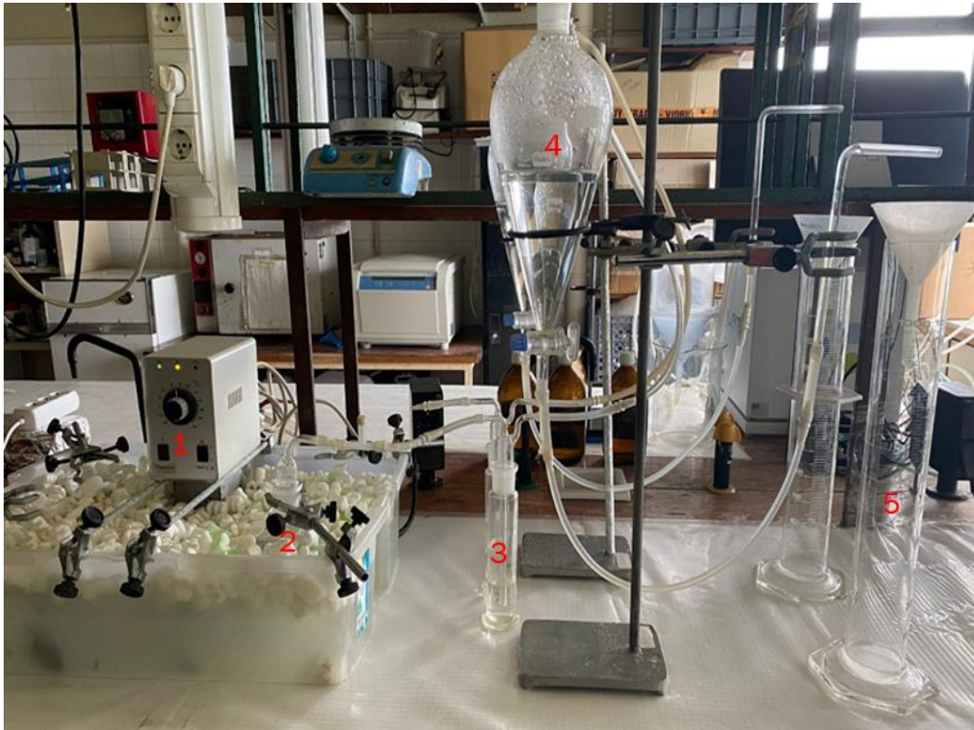
Figure 2 - Experimental set-up. 1-thermostat, 2-reactor inside water bath, 3-bubbler, 4-separating funnel, 5- graduated cylinder
