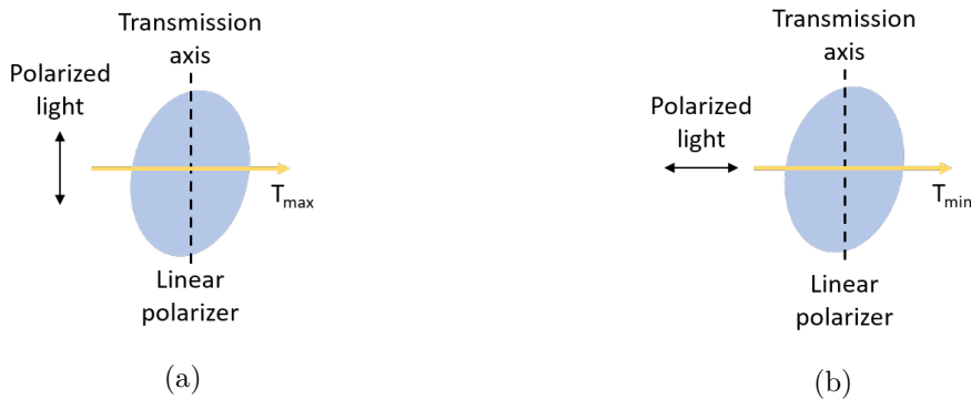
Figure 3.3: Schematic representation of the transmittance of a polarizer: (a) when the polarization of the incident light is parallel to the transmission axis of a LP the transmittance at the output is maximized; (b) when the polarization of the incident light is perpendicular to the transmission axis of a LP the transmittance at the output is minimized.
