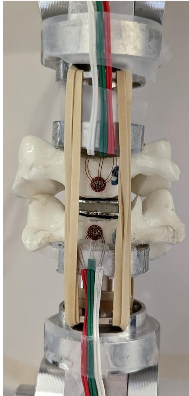
Figure 3.9 Experimental assembly with the prosthetic disc placed between the vertebrae.
