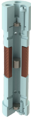
Figure 2.3: Schematic representation of the electromagnetic harvester proposed by Santos et al. [4].
