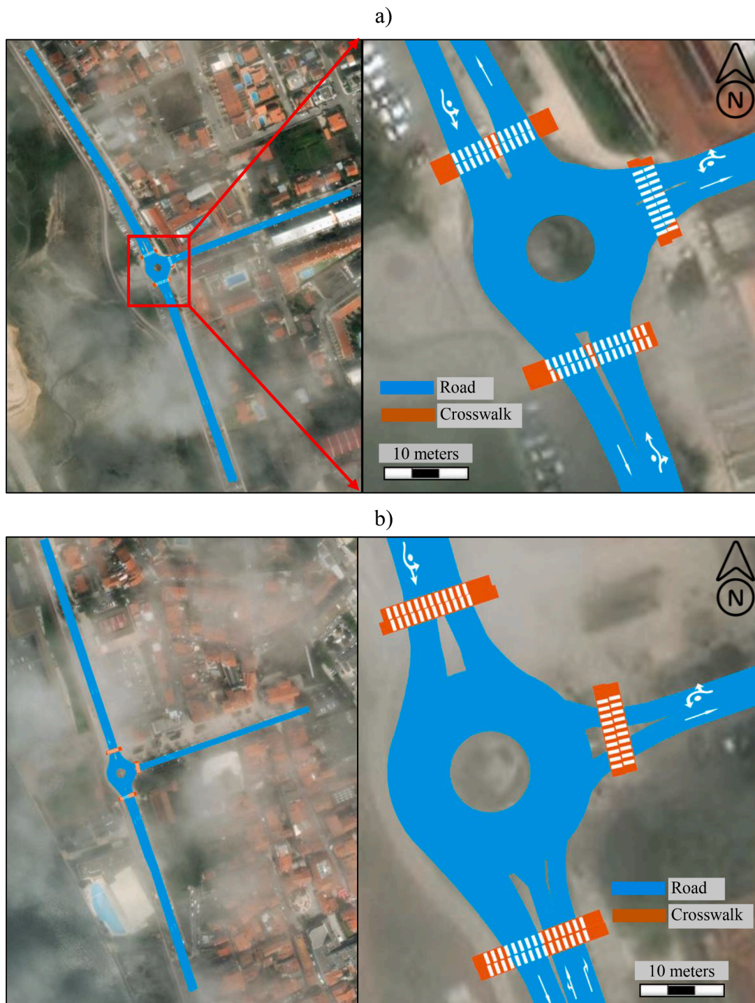
Fig. 7. VISSIM models for the studied single-lane roundabouts: (a) S1 and (b) S2. [Source: Bing Maps]
