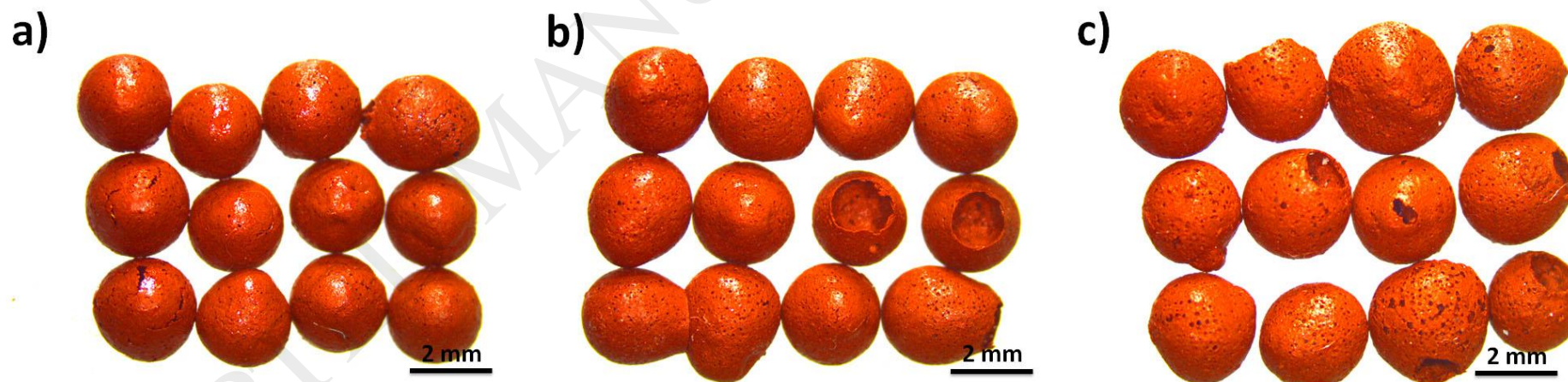
Fig. 5 Optical characterisation of the red mud-containing geopolymer spheres prepared with varying pore forming agent content: a) 0.30 g, b) 0.40 g and c) 0.59 g.
