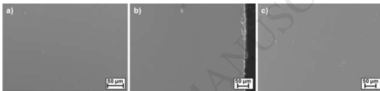
Fig. 2 Longitudinal section SEM micrographs (500X) of (a) LGSO-1, (b) LGSO-3 and (c) LGSO-5 fibres.
