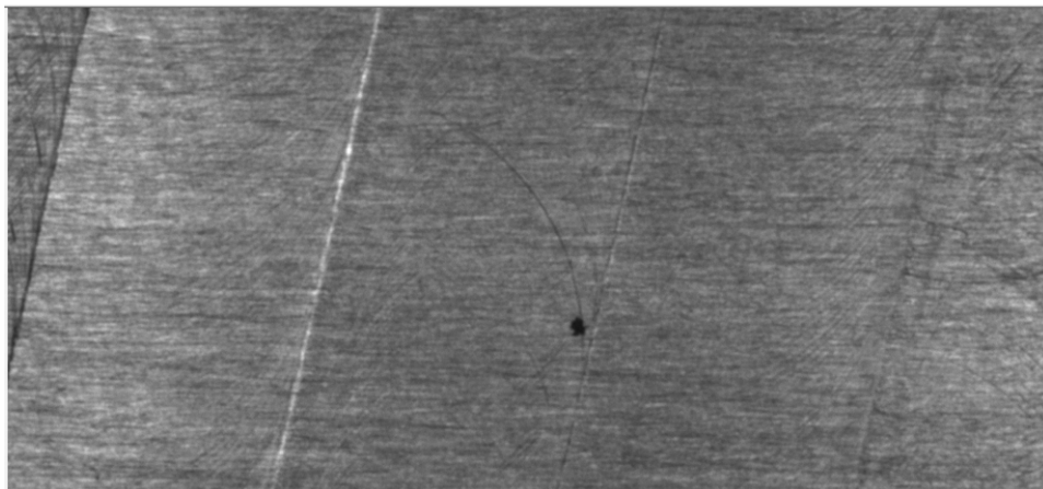
(b) Bloco 5 polido zona 2 ( R_a=0.442 e R_z=2.188 )
