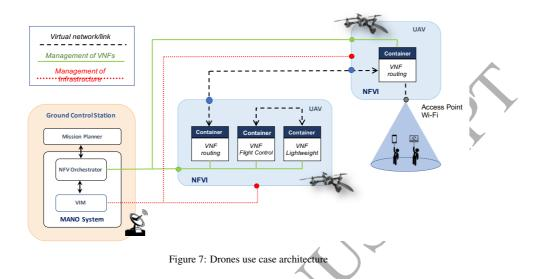
to the UAVs to enable the execution of lightweight VNFs. The lightweights VNFs are implemented using the containers as virtualization technology. This solution offers a more elastic way for implementing function virtualization in the UAS context, since the hardware and software resources provided by the UAVs is limited. The work in [14] presents the preliminary idea along with different experiments to validate the feasibility of a system like the already presented throughout this section.
