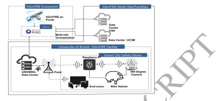
Figure 5: Smart City Safety experimentation architecture.
