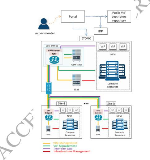
Figure 2: 5GinFIRE high level experimental architecture.
