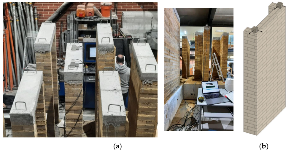
Figure 7. Dynamic identification test: (a) sensors placed during one setup and (b) axonometric scheme of the location of the sensors.
