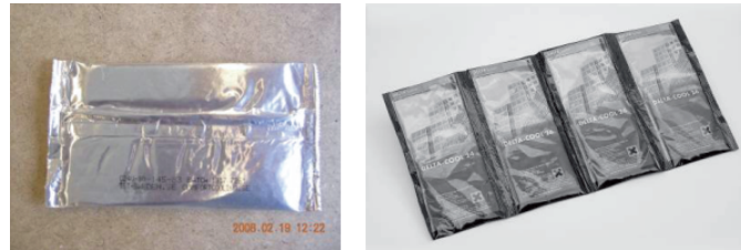
Figure 2.4: Examples of macroencapsulation; left produced by Climator, right produced by Dörken [4]
