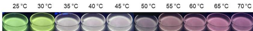
Figure 10 Pictures of 1@PMMA material deposited on the top surface of glass under 366 nm irradiation at different temperatures.
