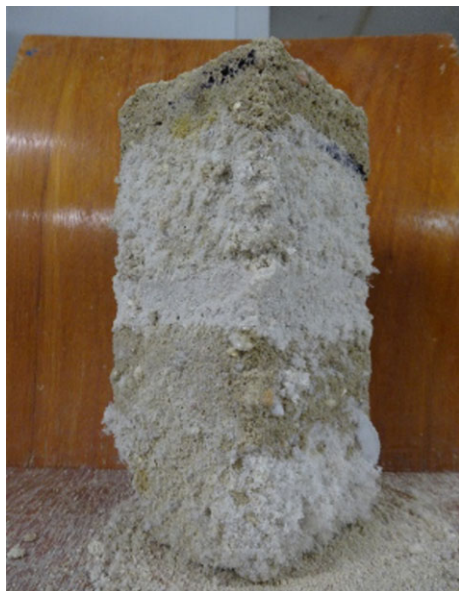
Fig. 14. Adobe combined block ( 18 \times 8 \times 8 \text{ cm} ) after capillarity test with aqueous solution of sodium sulfate 1.15 \text{ mol kg}^{-1} (© Alice Tavares).
