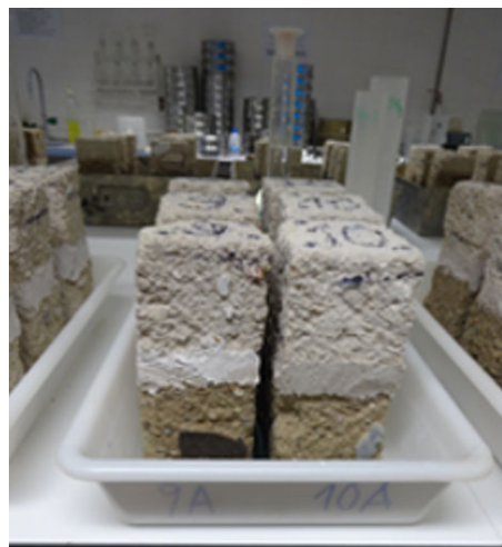
Fig. 8. Adobe combined blocks (18 × 8 × 8 cm) under capillarity test (© Alice Tavares).
