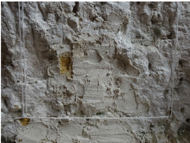
Fig. 16. Sacrificial mortar on formed wall. Sampling sites are the yellow areas, grid size – 50 × 40 cm (© Alice Tavares).
