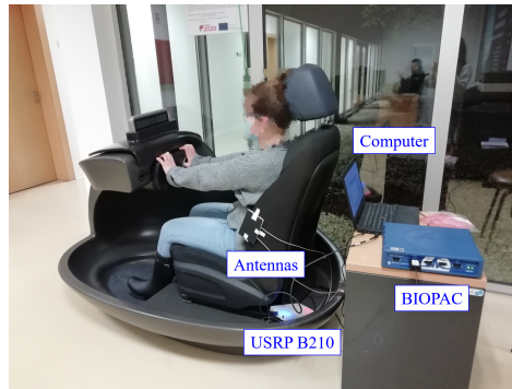
Figure 4.35: Setup used in the vital signs acquisition for the final upholstery prototype validation.
