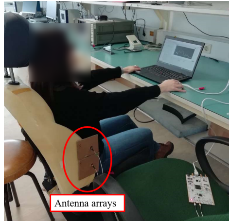
Figure 4.22: Position of the LHCP and RHCP antenna arrays in the car seat to acquire respiratory signals.
