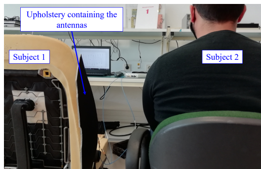
Figure 4.32: Setup used to test the effectiveness of the antenna insulation.
