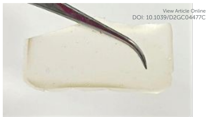
Fig. 6 Keratin film processed from chicken feathers waste.
