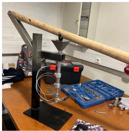
Figure 66 Injection machine without electrical box.
