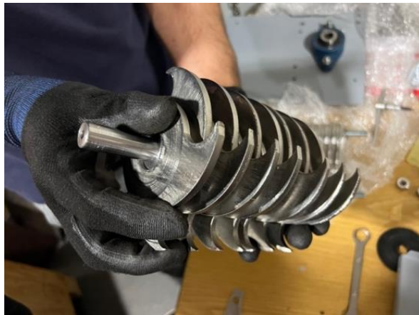
Figure 42 Assembled the main shaft.
