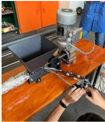
Figure 57 Plug-in connectors in place.
