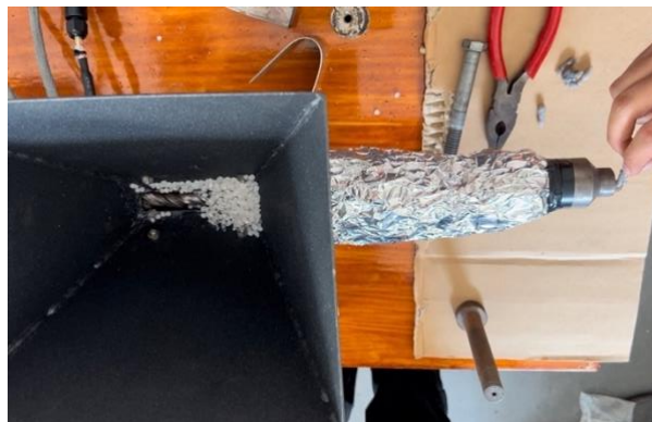
Figure 61 Material (HDPE) in the nozzle.
