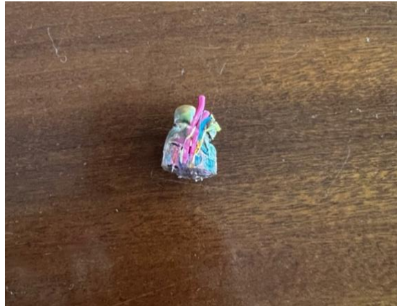
Figure 72 Result of PLA in the injection machine.
