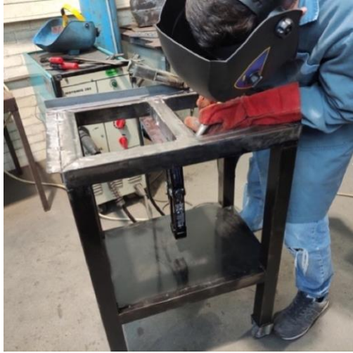
Figure 75 Welding of carjacking in base and correction of measurements in the top part.
