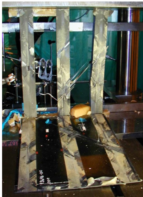
Figure 8. Multiple stiffeners debonding from a panel under compression [1] (courtesy of Ministry of Defence)
