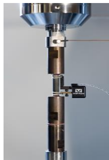
Figure 1. Set-up of cyclic tensile tests.
