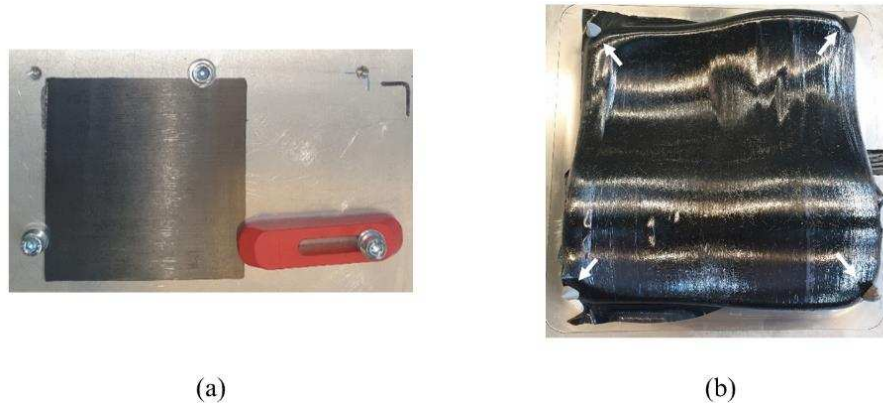
Figure 2. (a) Top view of the [0^\circ]_4 CFEP-plate (fixed on three points for the FScan) and (b) manufactured double sine geometry with plasticine markers
