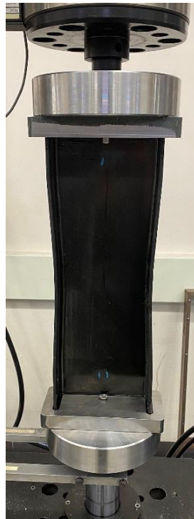
Figure 5: C-spar mounted in hydraulic test machine
