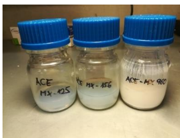
Figure 1. 25 wt.% concentrate of CSR particles ACE MX-125, MX-156 and MX-960 in the epoxy.
