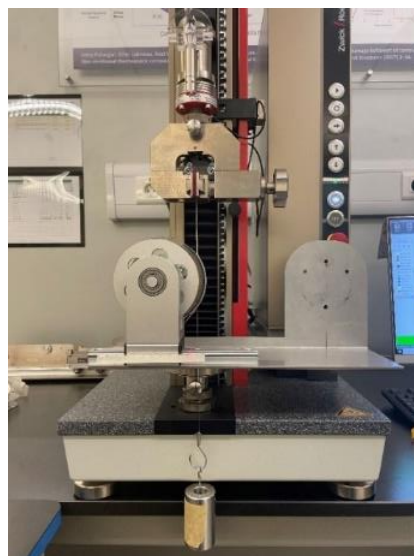
Figure 3. The prototype of the cassette-like peeling system.
