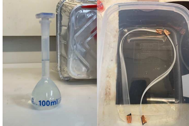
Figure 1. Silane solution (left), immersed fibre bundles in the silane solution (right)
