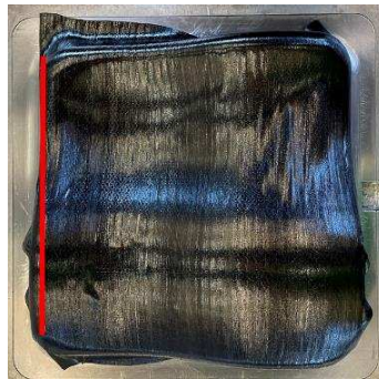
Figure 6. Reference line definition for the double sine geometry
