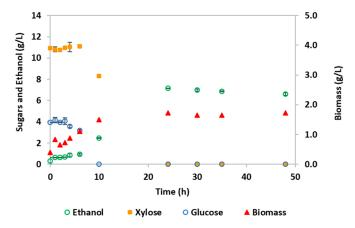
**Figure 3.** Time course of *E. coli* MS04 fermentation using the hydrolysate detoxified by membrane nanofiltration: glucose, xylose, bioethanol and biomass concentrations (45 mL, 150 rpm, initial pH 7 and 37 °C).
