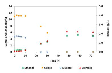
**Figure 1.** Time course of *S. stipitis* fermentation using the hydrolysate detoxified by membrane nanofiltration: glucose, xylose, bioethanol and biomass concentrations (50 mL, 150 rpm, initial pH 5.5 and 30  $^{\circ}$ C).
