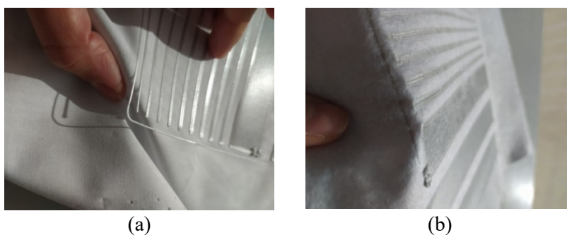
Figure 4. (a) Lack of adherence on the 65% polyester plus 35% cotton fabric. (b) Adherence showed on polyester felt fabric.
