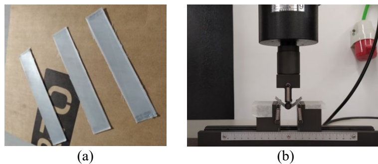
Figure 2. (a) 150 mm by 25 mm specimens. (b) Three-point Bending test.
