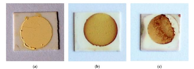
**Figure 2.** Optical images of  $TiTe_3O_8$  films deposited on carbon coated  $25.4 \times 25.4 \times 0.0254 \text{ mm}^3$  alumina substrates and sintered at 680 (a), 700 (b) and 720 °C (c) for 5 h, respectively. Films sintered at 680 °C are not fully dense and some films sintered at 720 °C exhibit an irregular surface with a reddish colour resulting from a reaction with the alumina substrate.
