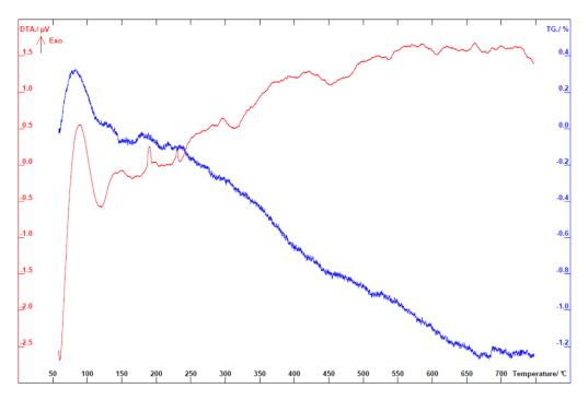
**Figure A1.** Differential thermal analysis (DTA) and thermogravimetric (TG) analysis curves recorded in air on graphite coated Al<sub>2</sub>O<sub>3</sub> substrate.
