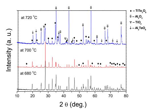
**Figure 3.** XRD patterns of TiTe<sub>3</sub>O<sub>8</sub> films deposited on carbon coated alumina substrates and sintered at 680, 700 and 720 °C for 5 h. The main film's phase is TiTe<sub>3</sub>O<sub>8</sub>. For films sintered above 700 °C Al<sub>2</sub>TeO<sub>6</sub> is formed due to a reaction between TeO<sub>2</sub> and Al<sub>2</sub>O<sub>3</sub> substrates.
