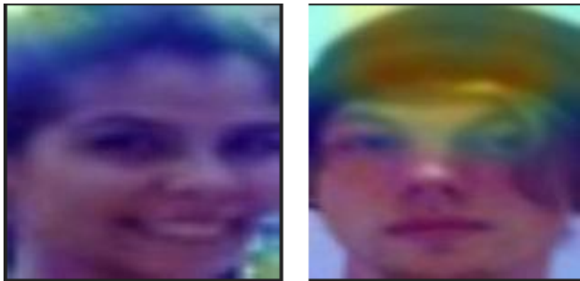
Figure 6.8: Averaging of Attention Maps for Hats Detection using the “handmade” VGG16 model with Koncept224 and cropping
