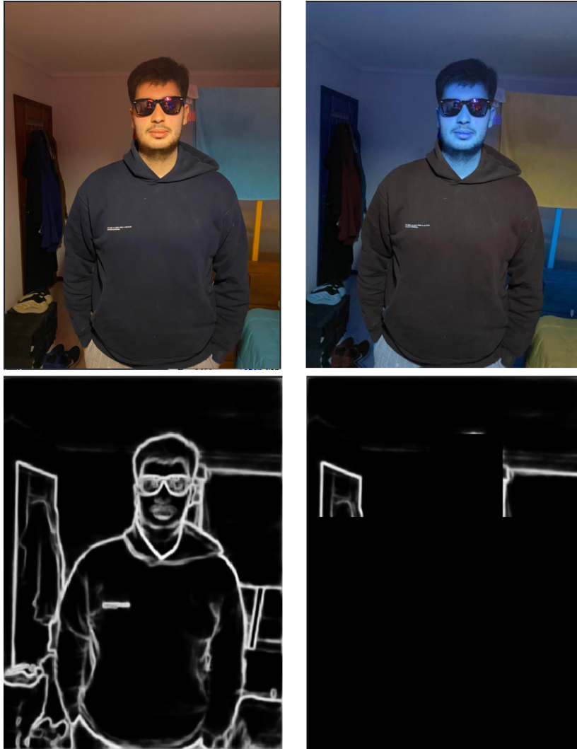
Figure 7.2: Preprocessing images steps of the Foresty tilt algorithm: Top-left - original image, Top-right - Rotated Image (RGB channels switched to acbgr), Bottom-Left - HED, Bottom-Right - HED without face region and all the region below mouth line
