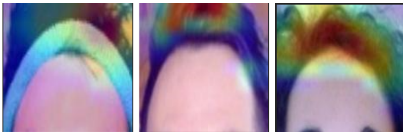
Figure 6.13: Examples of Bad Attention Maps for Hats Detection using the “handmade” VGG16 model with BRISQUE and head cropping
