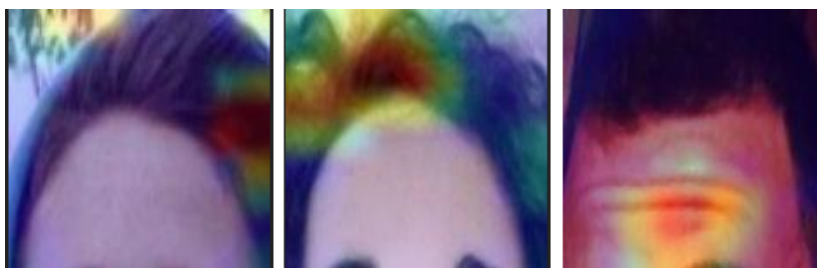
Figure 6.14: Examples of Bad Attention Maps for Hats Detection using the “handmade” VGG16 model with Koncept224 and head cropping
