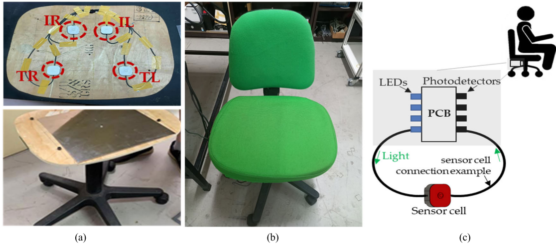
FIGURE 3. Office chair seat instrumentation process: (a) sensor cells installed on the wooden seat plate (top); aluminum plate fixed on the seat over the sensor cells (bottom); (b) finalized instrumented chair; and (c) schematic representation of sensor cell connection.
