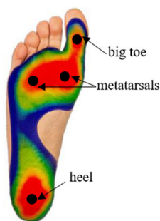
FIGURE 1. Typical plantar and shear forces distribution in the foot, with the areas with higher (red) and lower (blue) forces. Identification of the sensor-cells position (black dots).
