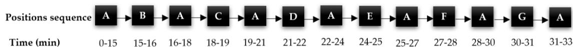
Figure 9. Scheme showing the sequence of pressure relief positions and their time at the first test.
