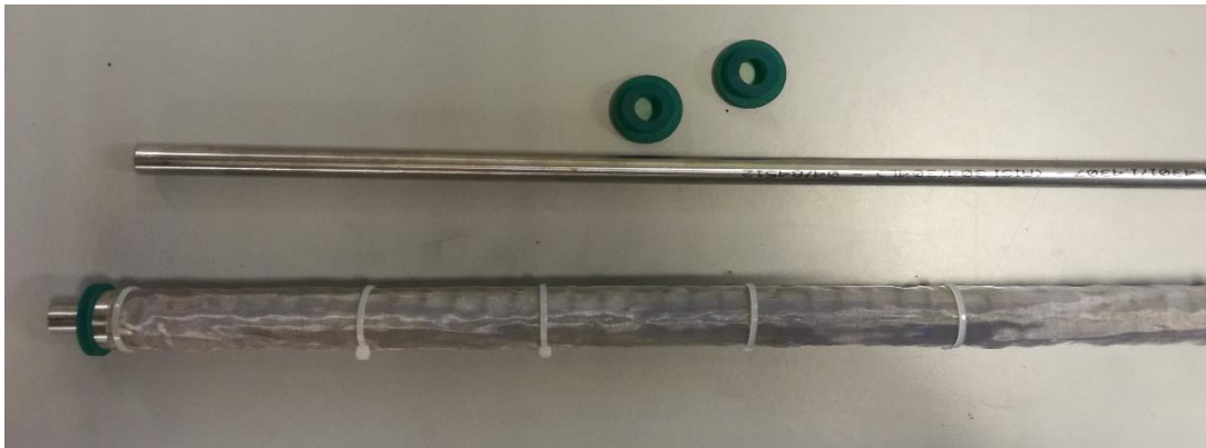
Figure 6.1 – Inner metal tube and an assembled adsorber tubular unit.
