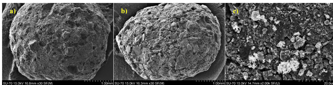
Figure 3.4-16: Microstructural evolution of the spent 50%C-Fe catalyst after the first (a) and third (b and c) gasification-regeneration cycle.
