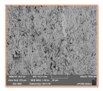
Fig 2 : Morphologic of surface on HCl (1M) + inhabit 14 day
