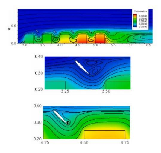
Fig 1 Streamlines and isotherms field for Re = 500.
