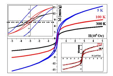
**Figure 1**: Magnetization hysteresis loops of radiation-induced Fe<sub>3</sub>O<sub>4</sub> nanoparticles at T = 5, 100 and 300 K. Insets: Left) Magnification of the low field region; Right) Modified Langevin in red function fit.
