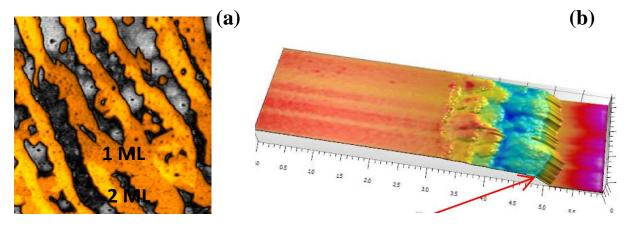
a) HD-KFM image on Graphene b) HD-KFM image of a cleaved perovskite solar cell.
