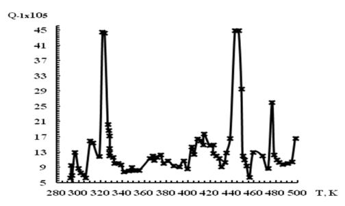
**Figure 1 -** Temperature dependence of internal friction  $Q^{-1}(T)$  in SiO<sub>2</sub>/Si wafer-plate ptype, doped with B, KDB-7.5(100) diameter  $D \approx 76 \cdot 10^{-3}$  m, thickness  $h_{Si} \approx 460 \cdot 10^{3}$  nm with SiO<sub>2</sub> layer thickness  $h_{SiO2} \approx 100$  nm after electron with energy  $W \approx 1,5$  MeV irradiation with energy  $W \approx 1,5$  MeV dose  $D_{e-} \approx 10^{14}$  cm<sup>-2</sup>
