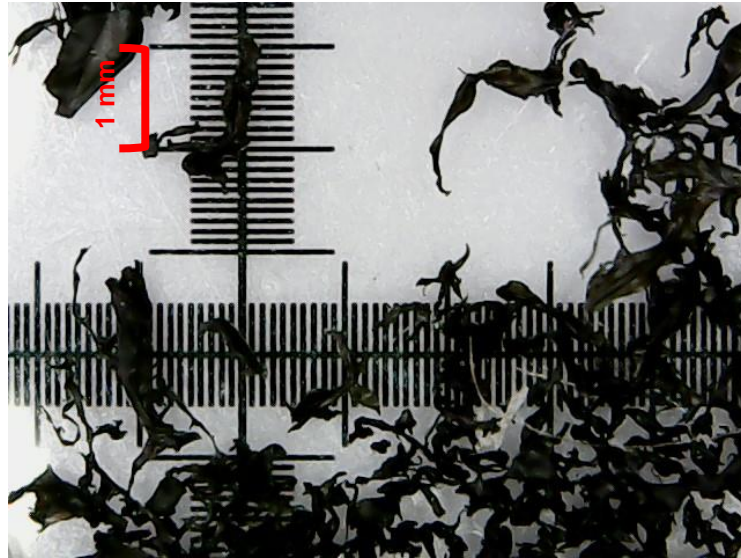
Figure 2.4. Variety of microplastic morphologies, which could lead to different rates of degradation, on a millimetric scale.
