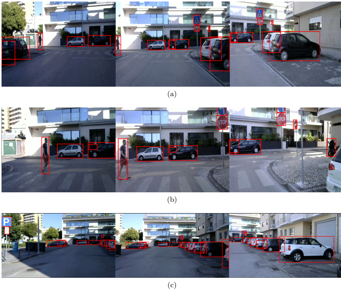
Figure 4.52: Inference on three video streams simultaneously. Each image (a),(b) and (c) represent a rendered tiled display with the three streams concatenated. Running at 12.5 FPS with YOLOR-CSP+NvDCF and detection interval of one.
