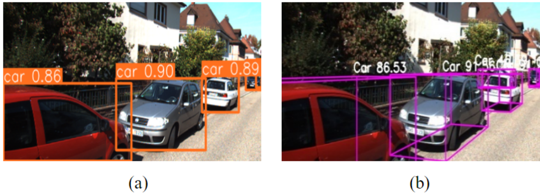
Figure 2.4: 2D vs 3D bounding box. [13]
