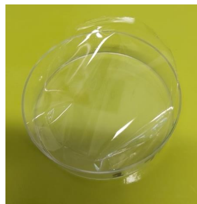
Figure 1. Representative photo of the biohybrid film doped with thulium triflate.
