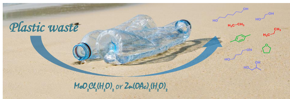
Scheme 1 – Reductive depolymerization of plastic waste catalyzed by cheap and environmentally friendly catalysts.
