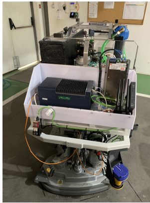
Fig. 2. Floor-cleaning robot prototype where the vision system was implemented and tested.
