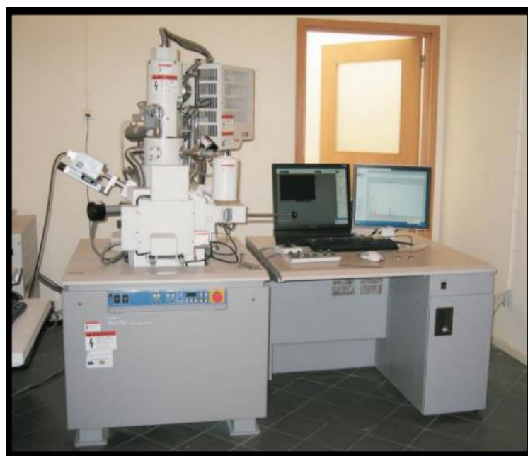
Figure 25 - Scanning electron microscope analysis (SU-70) used to collect the data.
