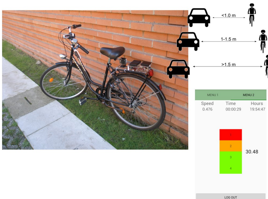
Figure 6 – On-board sensors platform for bicycles.
