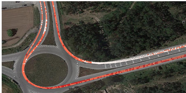
Figure 5 - Acceleration profile with In Car tracker. Red equals acceleration, white equals deceleration
