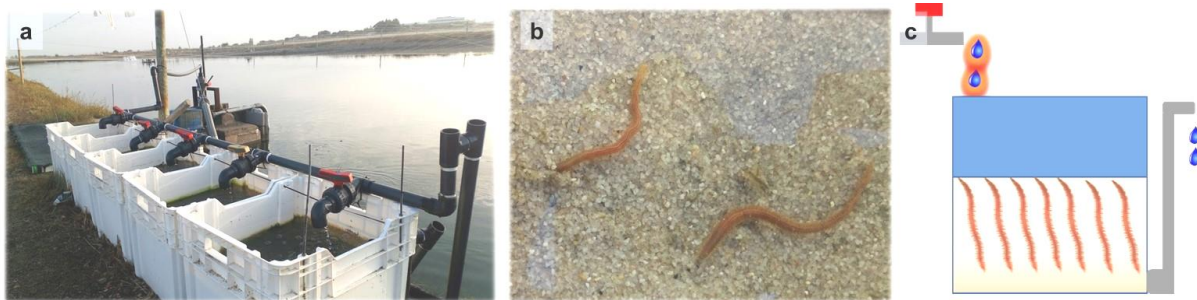
Figure 3.1. a) Polychaete assisted sand filters (PASFs) used in the present study; b) Hediste diversicolor in sand bed; c) Schematic representation of PASFs
