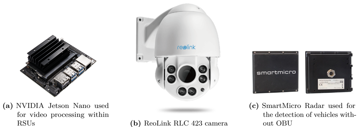
Figure 3.3: Computing and sensing equipment details
