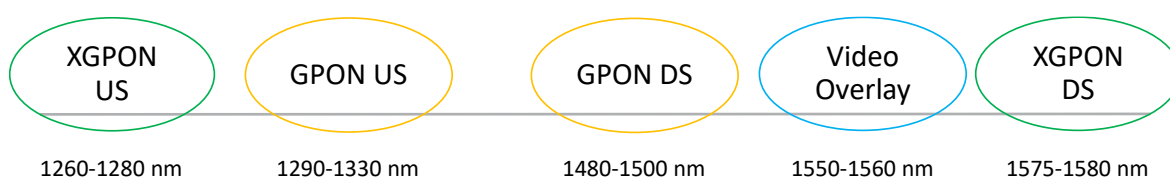
Figure 2-3 - Wavelength plan GPON, XG-PON, and video overlay.
