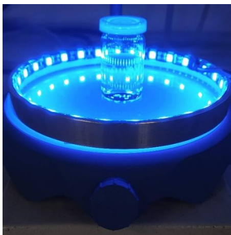
Figure III.2: Digital photograph of the blue LED light used in the experiments of the photocatalytic degradation of aqueous solutions of RhB and SMX.
