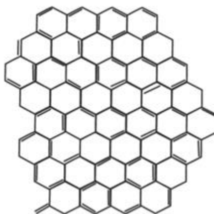
Figure 2 Graphene structure. Adapted from [19].
