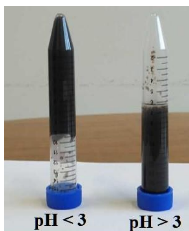
Figure S2.5 Photographs of the mixtures of the solutions of GO and PEI at pH below and above 3. The image shows that the formation of stable hydrogel between GO and PEI only occur for pH values lower than 3, where the electrostatic interactions are maximized.
