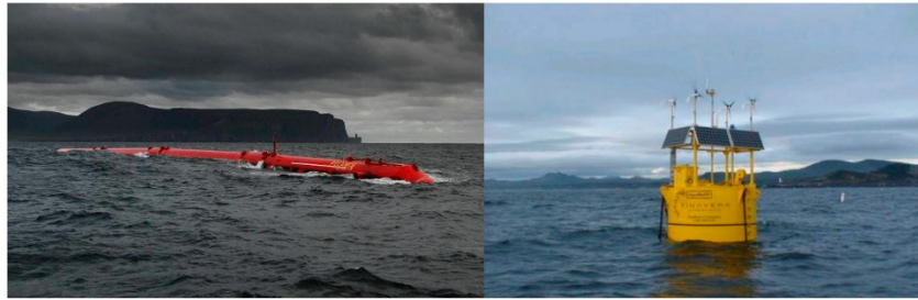
Figure 3.24 – The two WECs considered in this assessment: Pelamis (left) and Aqua Buoy (right). Image copyright from [173].
