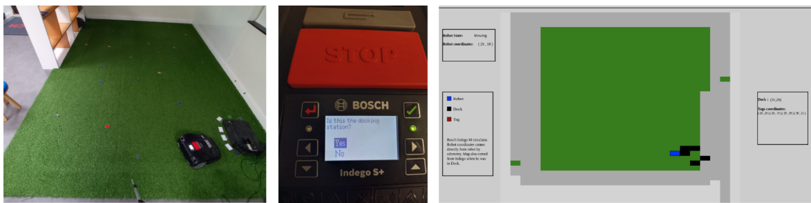
Figure 6.8: Dock identification with tags.
